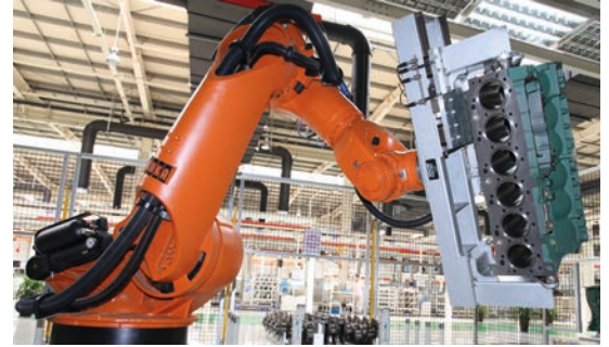
Gripping system for motor blocks (600 kg each) / loading and unloading of assembly stations
